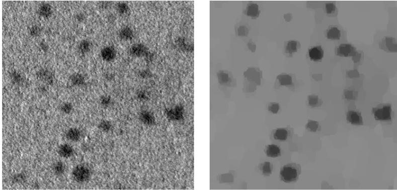
Image of silver nanoparticles (Silver proteinate, Fluka, Switzerland) before  $TV - L^1$  regularization and after it. Transmission electron microscopy images were provided by Anatolij Filimoněnko from IMG ASCR. Even the less contrast objects were preserved by the filtration and the resulting image is suitable for further processing and detection of particles by adaptive thresholding.
